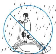
4. Do not ride your scooter in the heavy rain or wet conditions as this could damage the battery.
