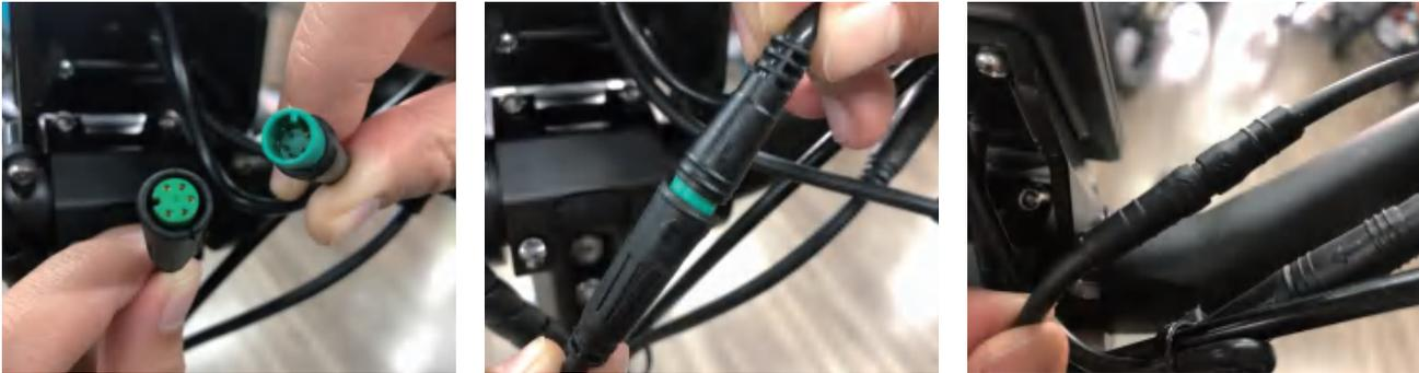
When connecting these two connectors, the arrow must be aligned with the arrow.
