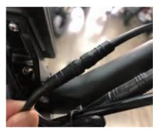
When connecting these two connectors, the arrow must be aligned with the arrow. You can turn on the power only when the assembly is completed.
